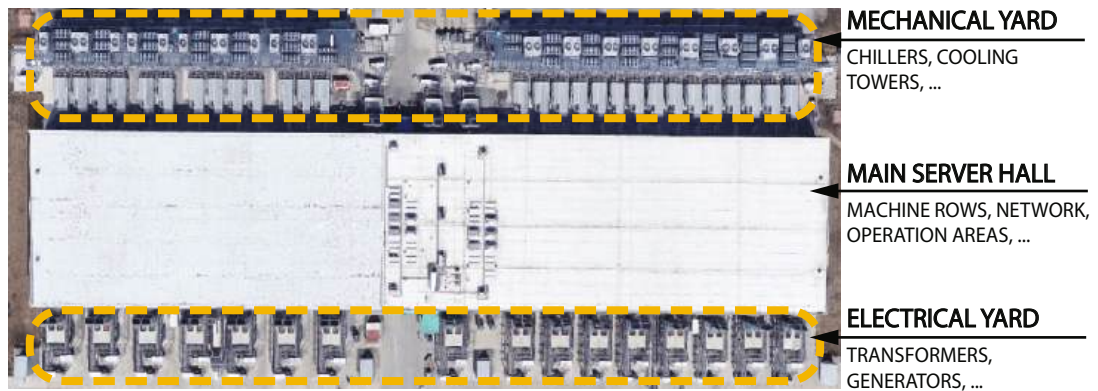
Figure 4.3: A Google data center building in Council Bluffs, Iowa, showing the mechanical yard, electrical yard, and server hall.
