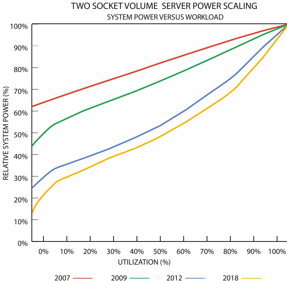
Figure 5.8: Normalized system power vs. utilization in Intel servers from 2007–2018 (courtesy of David Lo, Google). The chart indicates that Intel servers have become more energy proportional in the 12-year period.
