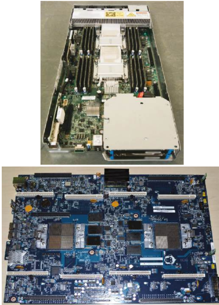
Figure 3.2: Example server trays: (top) Intel Haswell-based server tray and (bottom) IBM Power8-based server tray.
