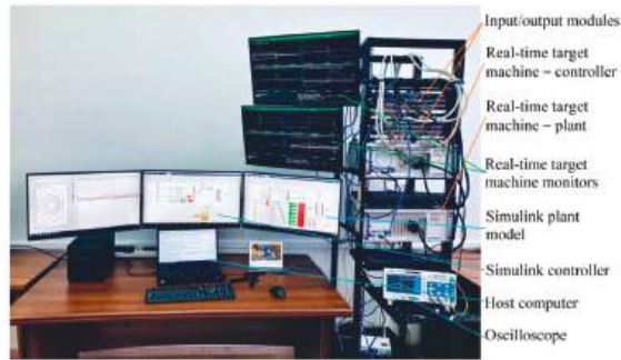
Figure 18. Real-time digital testbed at the V.A. Trapeznikov Institute of Control Sciences of the Russian Academy of Sciences.
