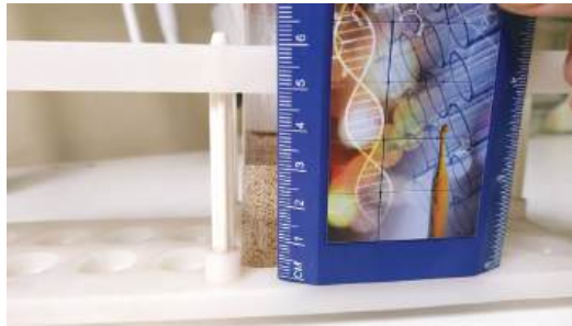
Figure 6. Determining the scale of the photograph by the size of the visible part of the test tube.
