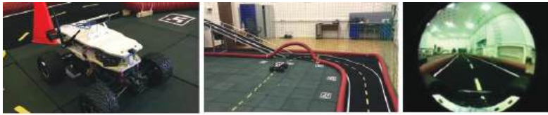
Figure 2. Landmarks in the form of yellow markings, red cones, and radio frequency markers.
