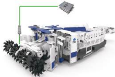
Figure 5. The vibration sensor location on bolter miner.
