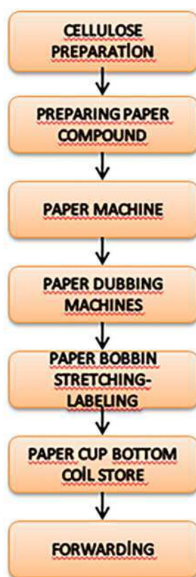
Figure 7.7 Pulp and paper manufacturing production processes.
