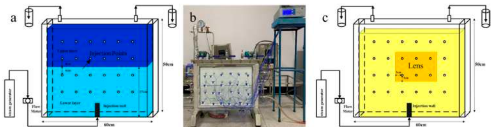
Figure 2. Schematic (a) and photo (b) of the experimental setup for the layered heterogeneous aquifer, and schematic of the experimental device for the lens heterogeneous aquifer (c).
