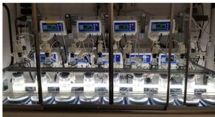
Figure 6.8 Photograph of S3 that can run nine parallel-fed batch bioreactors simultaneously.
