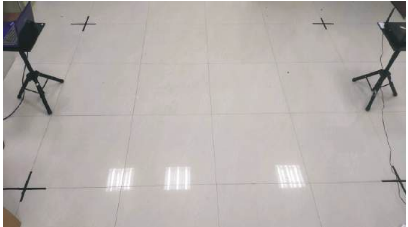
Figure 2. The area where the CSI data were collected. The crossbelt marks the boundary of the area, which is 2.4\text{ m} \times 3.2\text{ m} in size.
