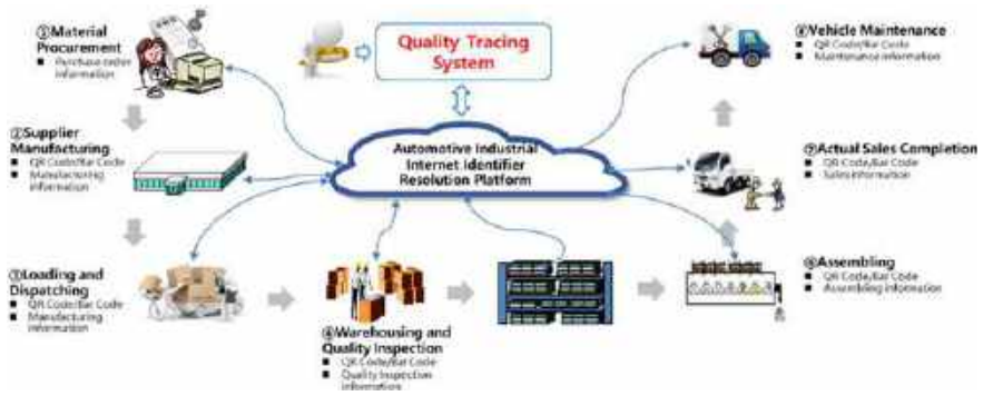
Fig. 5.37 Quality tracing based on identifier resolution [20]
