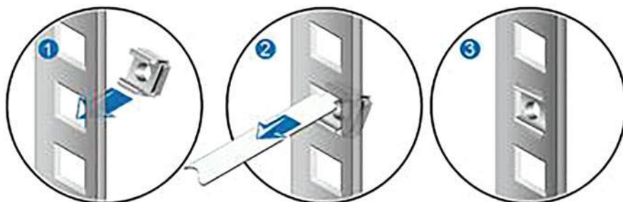
Fig. 3.105 Install the floating nut matched with the M6 screw
