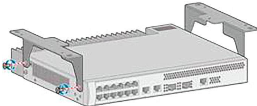
Fig. 3.69 Installation method of the ceiling-mounting ears
