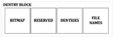
Fig. 3.14: F2FS Dentry Block Structure
