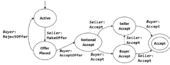
Fig. 3: The AssetTransfer state machine. The dashed arrow indicates a buggy state transition.
