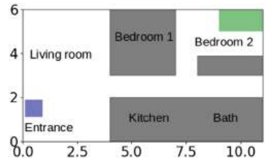
Fig. 1. The settings for controller synthesis of a mobile robot with reach-avoid specification.
