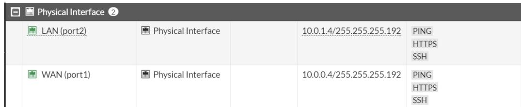
Figure 10.50: Firewall interfaces
