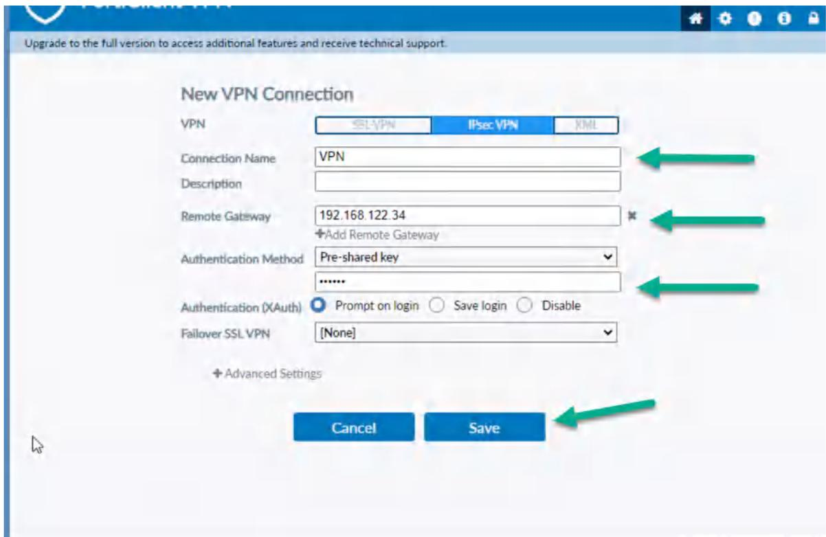
10. *Figure 4.23: Configure FortiClient Remote Gateway and Pre-shared key*
