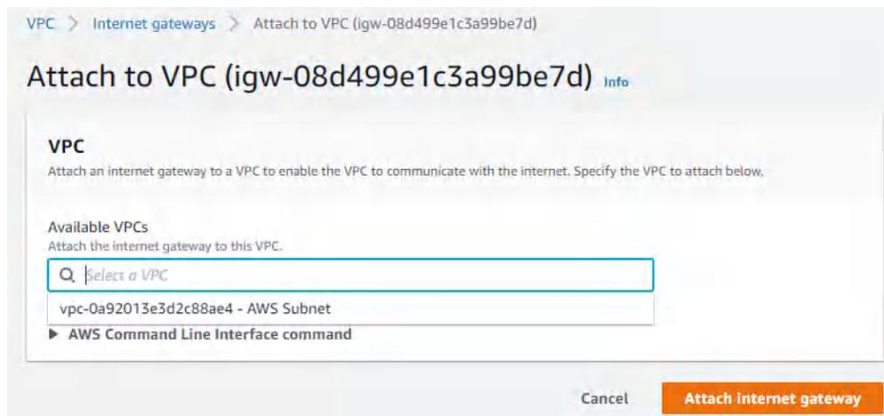
Figure 10.67: Attach the internet gateway to VPC
