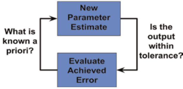
Figure 17. Cyclical process of deterministic parameter tuning.
