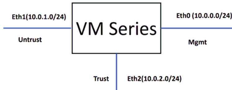
Figure 4.57: Palo Alto Firewall Interfaces by default
