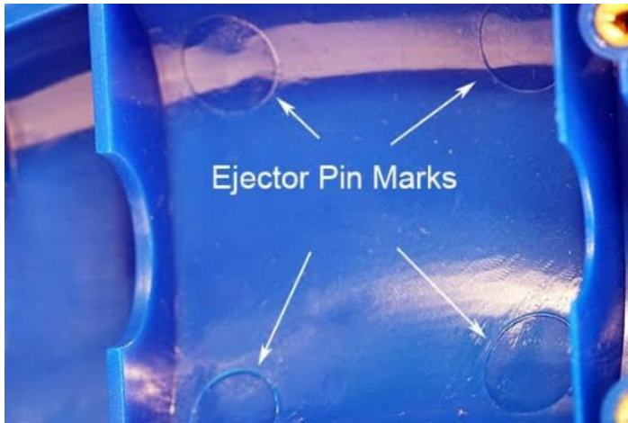
Ejector pin marks on a plastic housing part.
