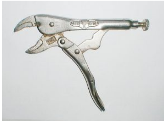
Vice grip or locking pliers are an example of a non-Grashof linkage that utilizes the toggle position for functionality.
