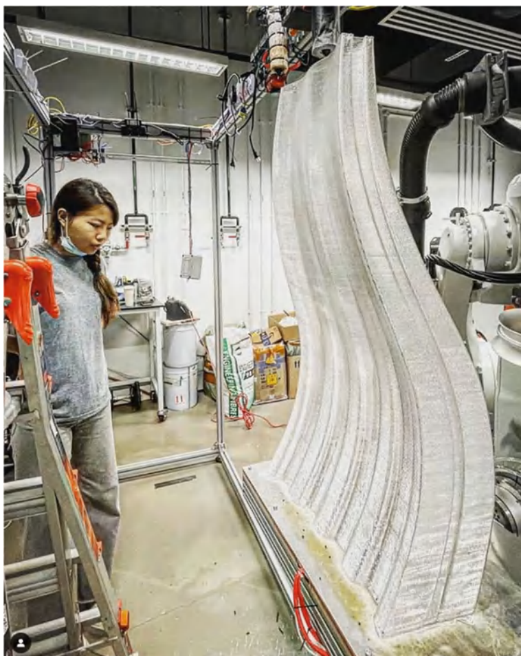
Fig. 5. Printing process for a large piece of the dome. The 1.5 m tall piece is almost complete. The Robot positions a heated built plate (bottom of the image), while the extruder is stationary on a frame (top of the image).
