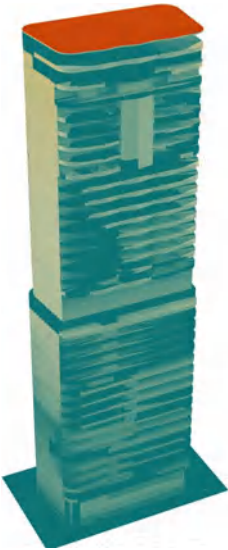
Fig. 7. Grasshopper/Rhino 3d definition showing environmental analysis. Relative humidity Each colour represents a different microclimate. The colours result from the cross-reference between the environmental analysis and the microclimate parameters. (3D image by author)
