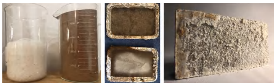
Fig. 3. Sodium Thiosulphate, Dune sand brick “growing”, final sodium sand brick.
