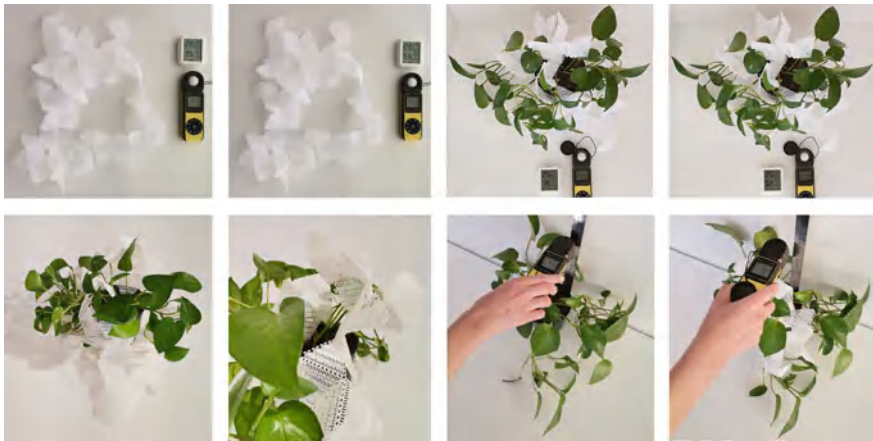
Fig. 6. Photos of the structures without water (39% of humidity) and with sprayed water (53% of humidity); structures arranged around a plant without water (39% of humidity) and with sprayed water (62% of humidity); photos of the structures arranged around a plant; the amount of lux was measured just on a plant (44.5 lux) and subsequently on the structures arranged around the plant without water (78.5 lux).
