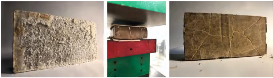
Fig. 4. Salt brick, compression test & resultant brick.
