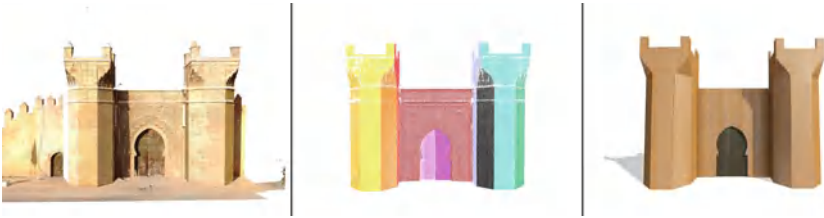
Fig. 6. Three stages of Chellah's gate reconstruction.
