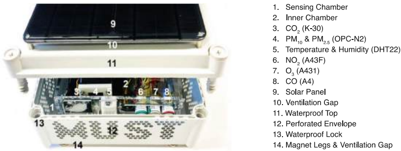
Fig. 3. MUST sensing kit configuration.
