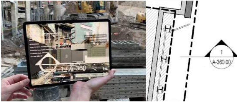
Fig. 3. Left, a screenshot of an interactive section cut callout in AR. Right, the counterpart call-out on within the traditional drawing set.
