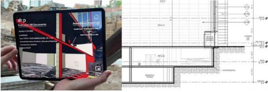
Fig. 4. Left, a screenshot of the section cut interactive BIM model in AR. Right, the counterpart section cut drawing within the traditional drawing set
