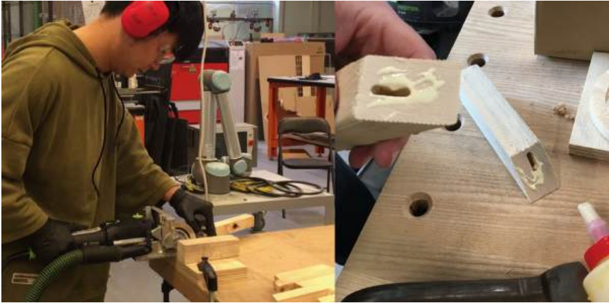
Fig. 5. A standardized timber domino system was used to fix the parts of the aggregation together
