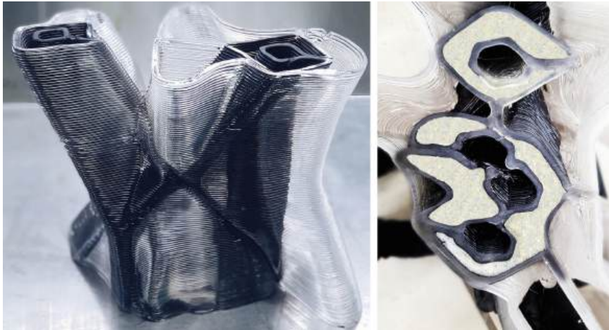
Fig. 5. 3F printed sacrificial formwork (left), preparation for carbon infusion (right)
