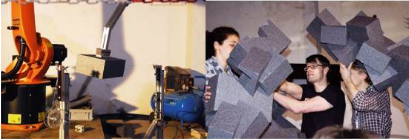
Fig. 3. Robot arm hot-wire cutting process (left) and result (right).
