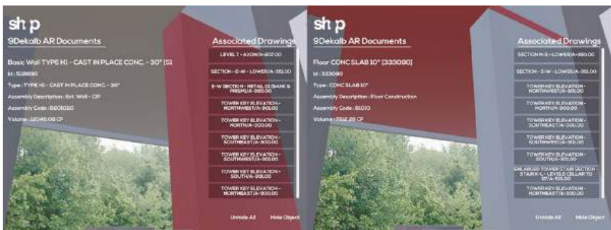
Fig. 2. A screenshot showing the information and associated views of a selected model element
