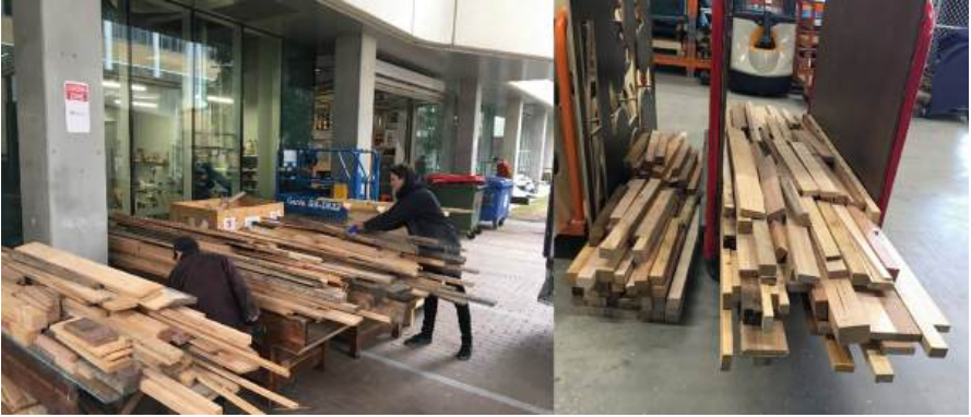
Fig. 1. A variety of timber offcuts categorized by their cross section profiles
