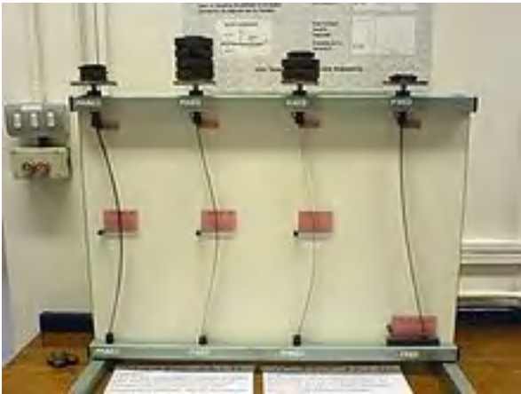
Figure 9.1.1 Types of buckling deformation (Wikipedia)
