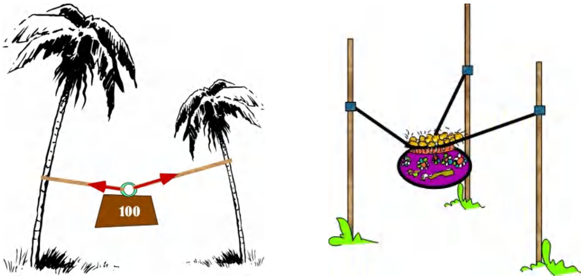
Figure 4.1 Suspended weight in two and three dimensions
