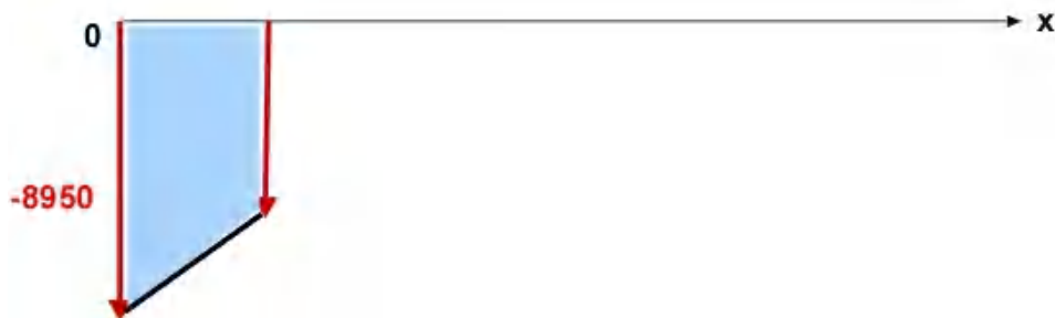
Figure 7.1.11a M(x) in Section AB
