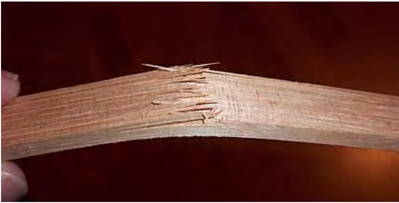
Figure 3.11.4 Failure in bending
