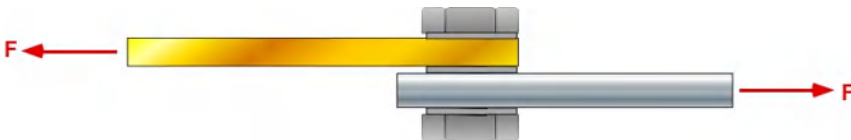
Figure 6.1.2 Bolt in single shear
