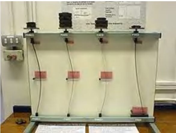
Figure 3.12.3 Types of buckling deformation (Wikipedia)
