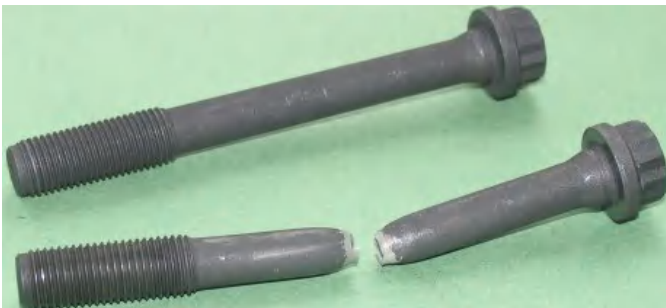
Figure 3.9.1 Failure in tension (necking)
