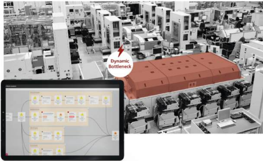
Fig. 4. Dynamic value stream and bottleneck analysis (IPSO Factory)
