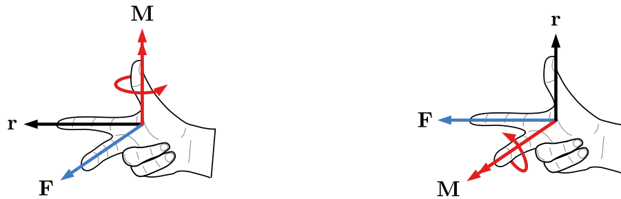
Figure 4.1.5 Three finger right-hand rule for moments.
