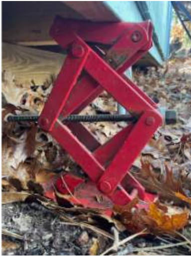
(a) A scissors jack uses fixed screw and a moving a nut.
