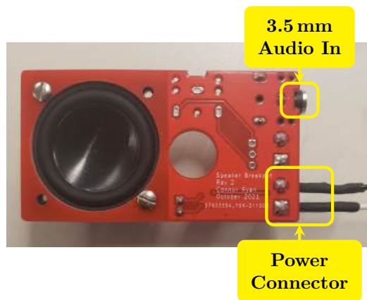
Figure 4.4: CyDAQ Speaker showing 3.5 mm Audio terminal and Power Connector .
