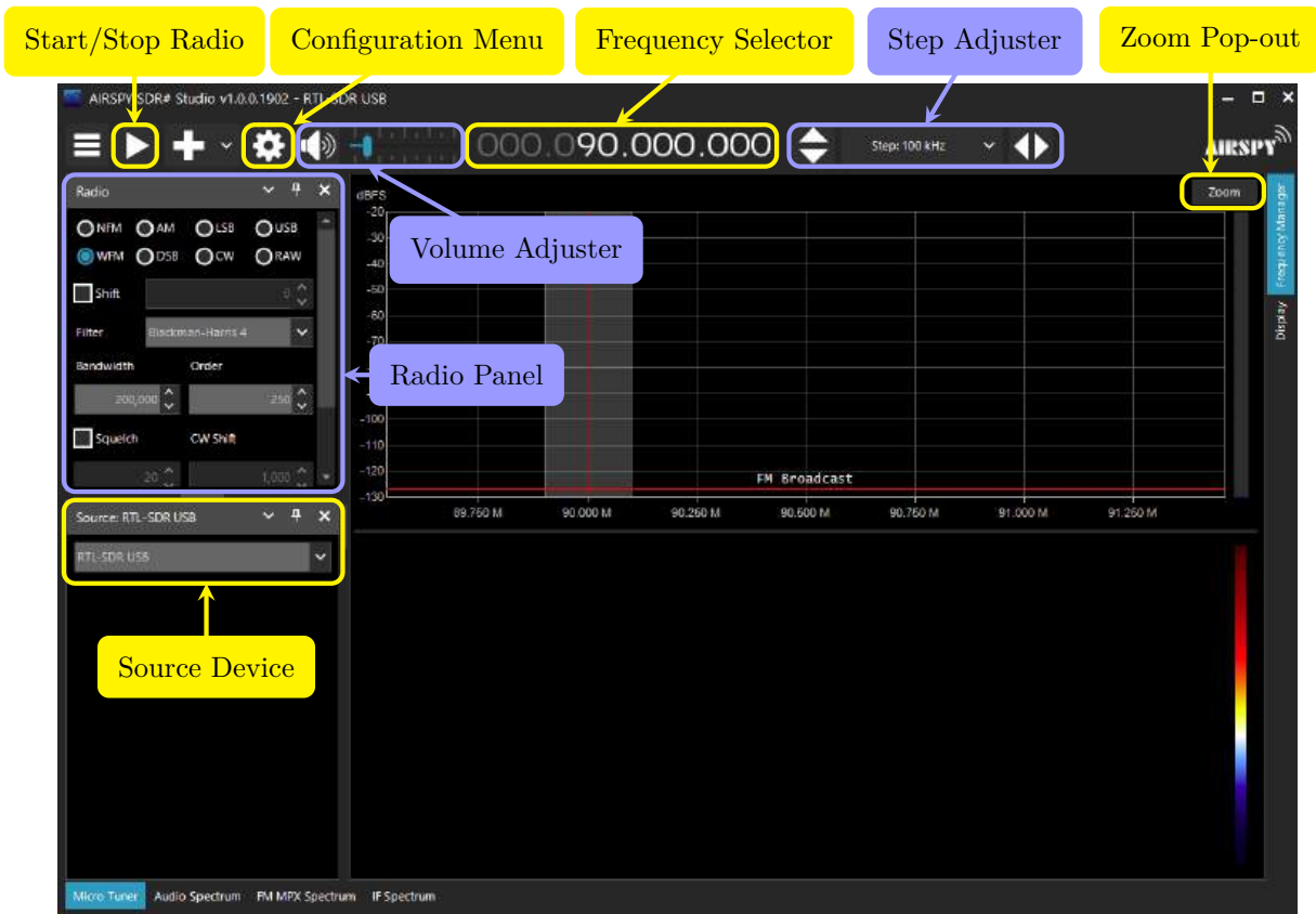
Figure 12.1: The SdrSharp Main Window with some of the less prominent features highlighted.
