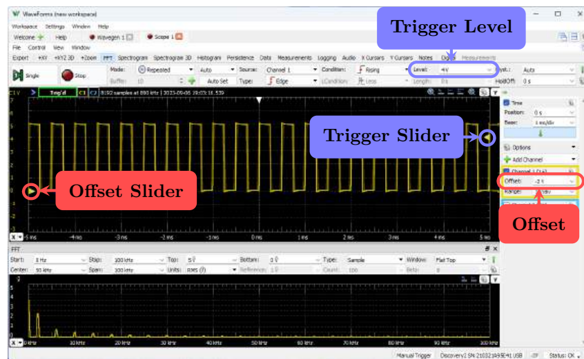
Figure 3.26: Scope with the Offset control, Offset Slider , Trigger Level control, and Trigger Slider highlighted.
