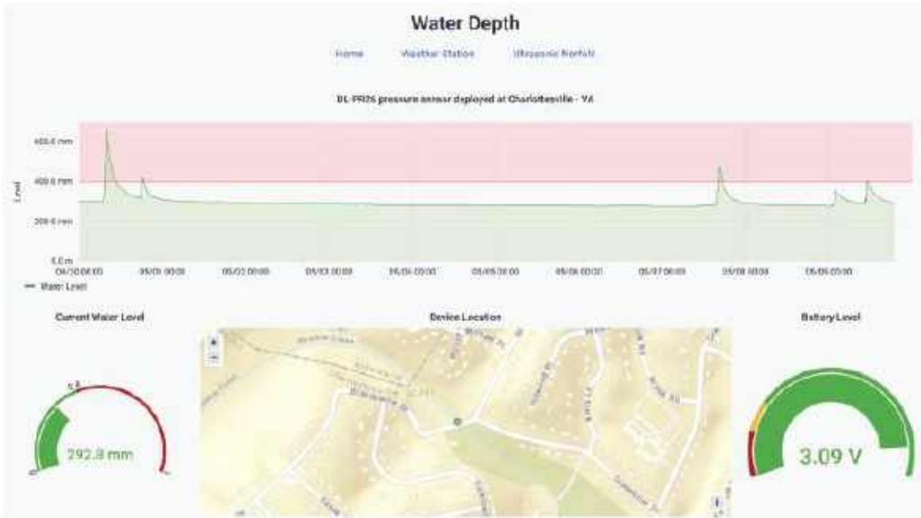
Figure 5. Grafana decision support dashboard of a water depth monitoring sensor.
