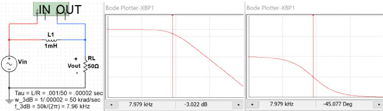
Figure 4.5: 1 st Order RL Low Pass Filter Circuit with a 3dB frequency ( f_{3dB} ) equal to 7.96 kHz.
