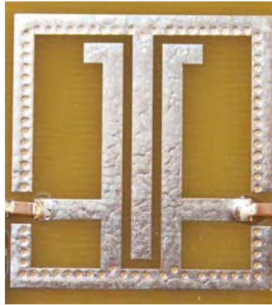
Figure 13.29: An L-band bandpass filter implemented using microstrip coupled resonators. The components on the left and right are surface mount capacitors, which are used to prevent DC shorting to ground.
