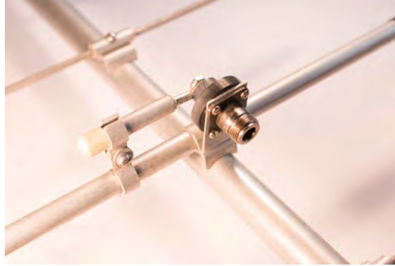
Figure 2.21: A gamma match used to interface coaxial cable to the driven element of a Yagi.
