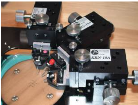
Figure 4-4: Micropositioners used with coplanar probes. Used with permission of J MicroTechnology, Inc.
