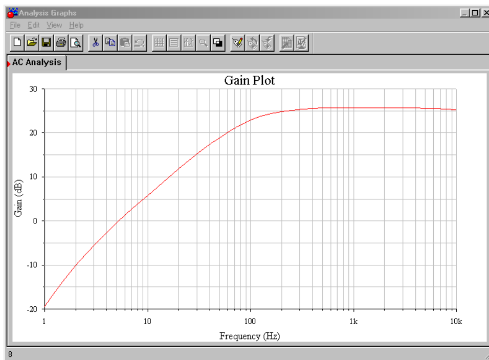
Figure 6.28b Gain plot for LM3900 amplifier.
