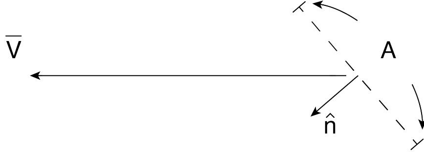
Fig 4.3 Flow through area A with outward normal \hat{\mathbf{n}} and velocity vector \bar{\mathbf{V}} .
