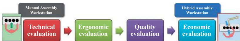
Fig. 12.3 General evaluation workflow and related priorities for the workstation transformation
