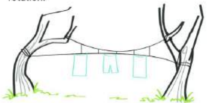
Adding a cable below can also stabilize the line and is more efficient
