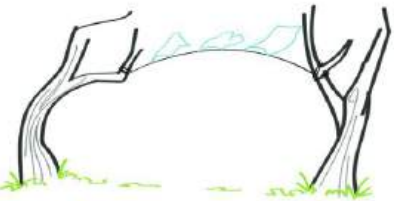
Clothesline: A steady flow of wind may cause clothesline to reverse the curvature
