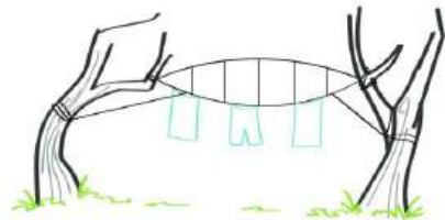
A second cable of reversed shape could be added above to retain the shape and resist upward loads. Stays are needed to prevent rotation.
