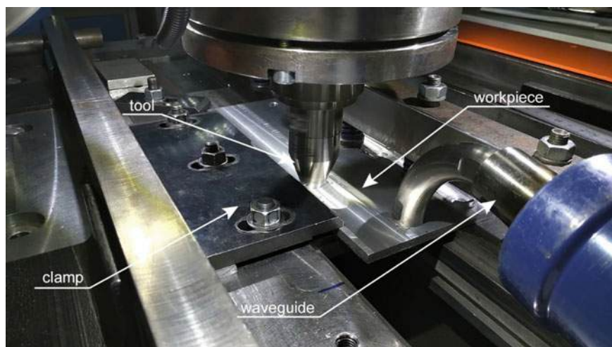
Fig. 6 Friction stir processing set up
