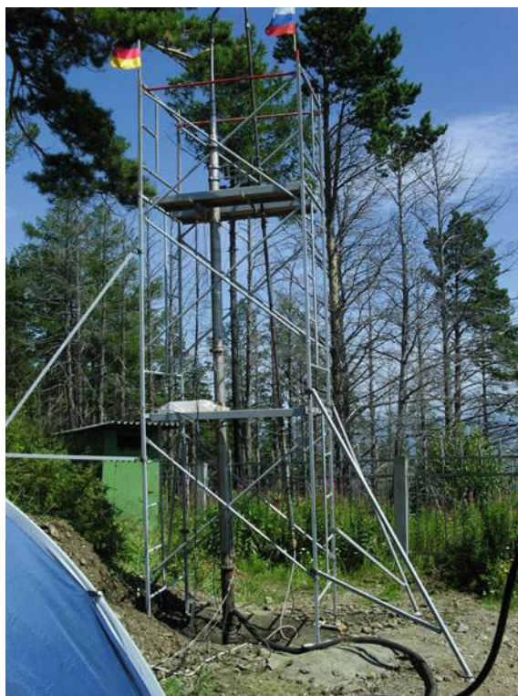
Fig. 1 The Borehole Generator of Seismic Waves (BGSW) mounted at one of the sides of the Angarsky fault
