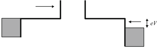
Fig. 16.3 Illustration showing the assumption that the charge reservoir on the right is shifted down by eV and that the electric field is not affecting the band structure of the system
