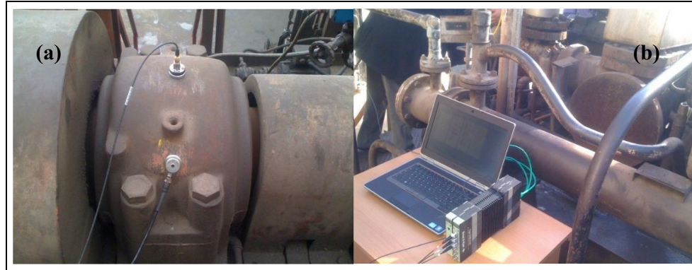
Figure 15. (a) Location of accelerometers and (b) pulse analyzer 16.I.
