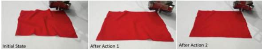
Fig. 11 Example of real fabric manipulation results. The figure shows three different steps during the manipulation following the actions suggested by the system. The sample manipulated is one from the real Use Case of the MERGING Project. In the figure, it can be clearly appreciated how the wrinkledness is reduced as the actions are applied
