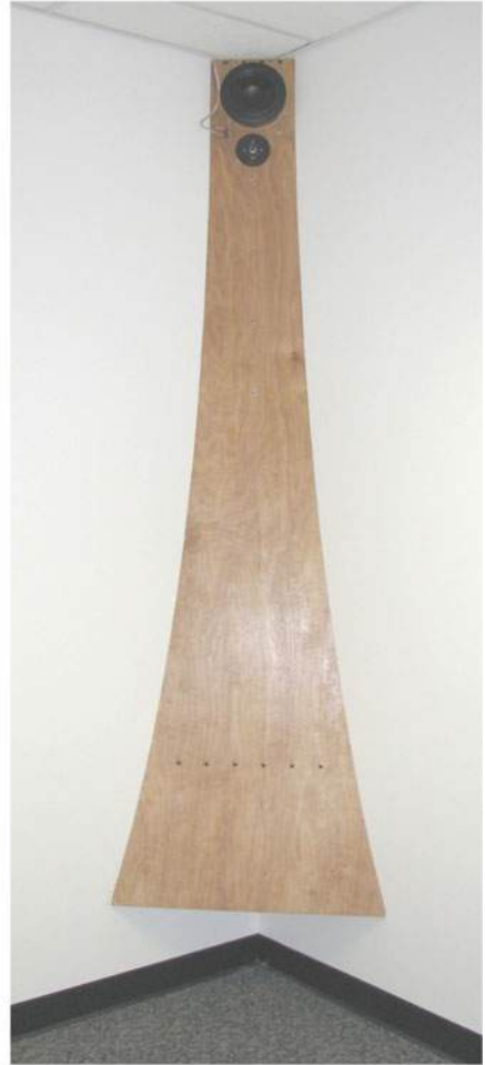
Fig. 10.21 (Right) Corner horn (this horn design, suggested by I. Rudnick, is particularly simple because it involves cutting a single sheet of plywood with a hand-held circular saw that has its blade set at 45^\circ , creating a smooth cut that will produce a leak-tight seal against the walls of a room. Even though the plywood is fairly thin ( 3/8'' \cong 9.5 mm), it produces a rigid boundary since it is curved initially along one axis making it very stiff against bending along an orthogonal direction. The plywood is held against the walls with a single turnbuckle anchored in the corner. The place where the turnbuckle should be attached to the plywood is found by applying force to one location that pushes the plywood smoothly against the wall. A horizontal “stringer” is then screwed and glued to the plywood to accept the hook. The stringer’s position is visible in Fig. 10.21 due to the six flat-head screws that can be seen forming a line about one-sixth of the way above the bell.) created by a single sheet of plywood that is cut to produce a catenoidal change in cross-sectional area from 173 \text{ cm}^2 at the top to 0.152 \text{ m}^2 at the opening over a length of 8' \cong 2.4 \text{ m} . (Left) Plots of the acoustic pressure (solid black line) that is in-phase with the volume velocity (dashed blue line) within the horn created when the speaker, at the throat, is driven with an electrical input of 10 \text{ V}_{\text{pk}} = 7.07 \text{ V}_{\text{ac}} . At x = 0 , the volume velocity is equal to that produced by the rear of the loudspeaker. From top to bottom: f_1 = 77 \text{ Hz} , f_2 = 139 \text{ Hz} , f_3 = 204 \text{ Hz} , and f_8 = 618 \text{ Hz}
