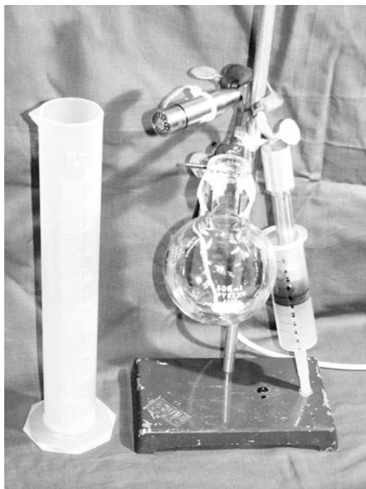
Fig. 8.16 Photograph of a 500 ml boiling flask and a B&K 1" microphone (Type 4144; S/N 473976) mounted on a ring stand. The resonance frequency was determined by blowing over the neck to excite the Helmholtz resonance and measuring the frequency of the microphone signal using an HP 3561A Spectrum Analyzer. The nominal volume of the flask is 500 \times 10^{-6} \text{ m}^3 . The diameter of the neck is D_{\text{neck}} = 25.0 \pm 0.1 \text{ mm} , so the neck's cross-sectional area is A = \pi(D_{\text{neck}})^2/4 = 490.9 \times 10^{-6} \text{ m}^2 . The length of the neck, as measured from the top of the lip to the first flare into the volume, is \Delta x_{\text{neck}} = 49.2 \text{ mm} . The temperature in the laboratory during measurements tabulated in Fig. 8.17 was 22.5^\circ \text{C} , corresponding to a speed of sound, c = 345 \text{ m/sec} . To the right and left of the ring stand are the graduated cylinder and the syringe used to measure the water added to the flask that varied the volume producing the data plotted in Fig. 8.17
