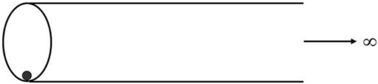
Fig. 13.29 Cylindrical waveguide with a source that is indicated by the solid black circle is located at an intersection of a rigid end cap and the cylindrical waveguide wall
