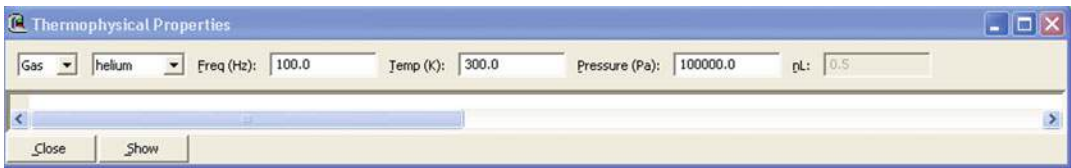
Fig. 8.18 Screenshot of the DELTAECS Thermophysical Properties window. The default material parameters are for 1 bar (100,000 Pa) helium gas at 300 K and an acoustic excitation at 100.0 Hz
