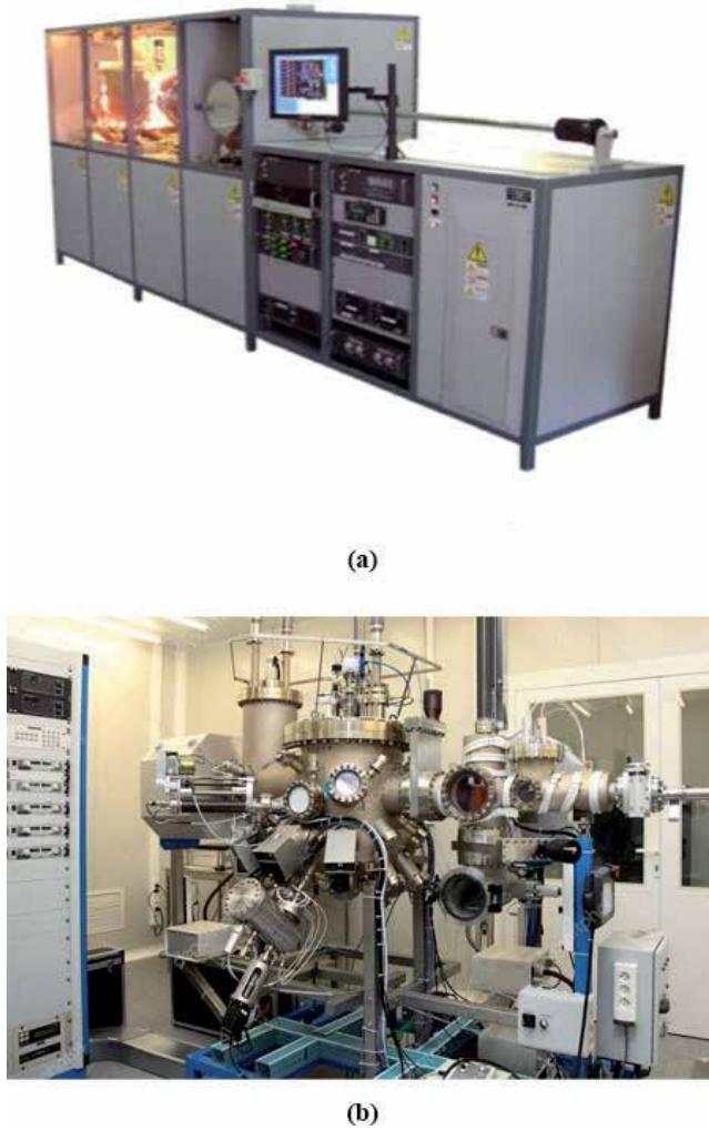
Figure 3. Photographs of (a) chemical vapor deposition (CVD) and (b) molecular beam epitaxy (MBE) systems (pictures were taken with permission from nanoscience Center, Cambridge, UK).
