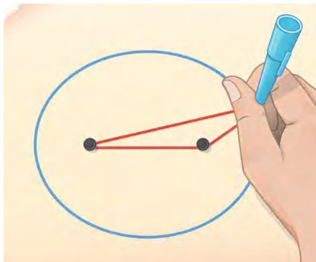
Figure 7.3 You can draw an ellipse as shown by putting a pin at each focus, and then placing a loop of string around a pen and the pins and tracing a line on the paper.
