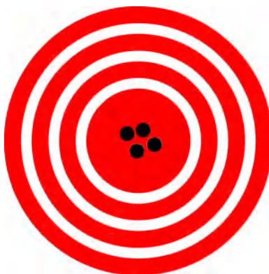
Figure 1.23 In this figure, the dots are concentrated close to one another, indicating high precision, but they are rather far away from the actual location of the restaurant, indicating low accuracy. (Dark Evil)
