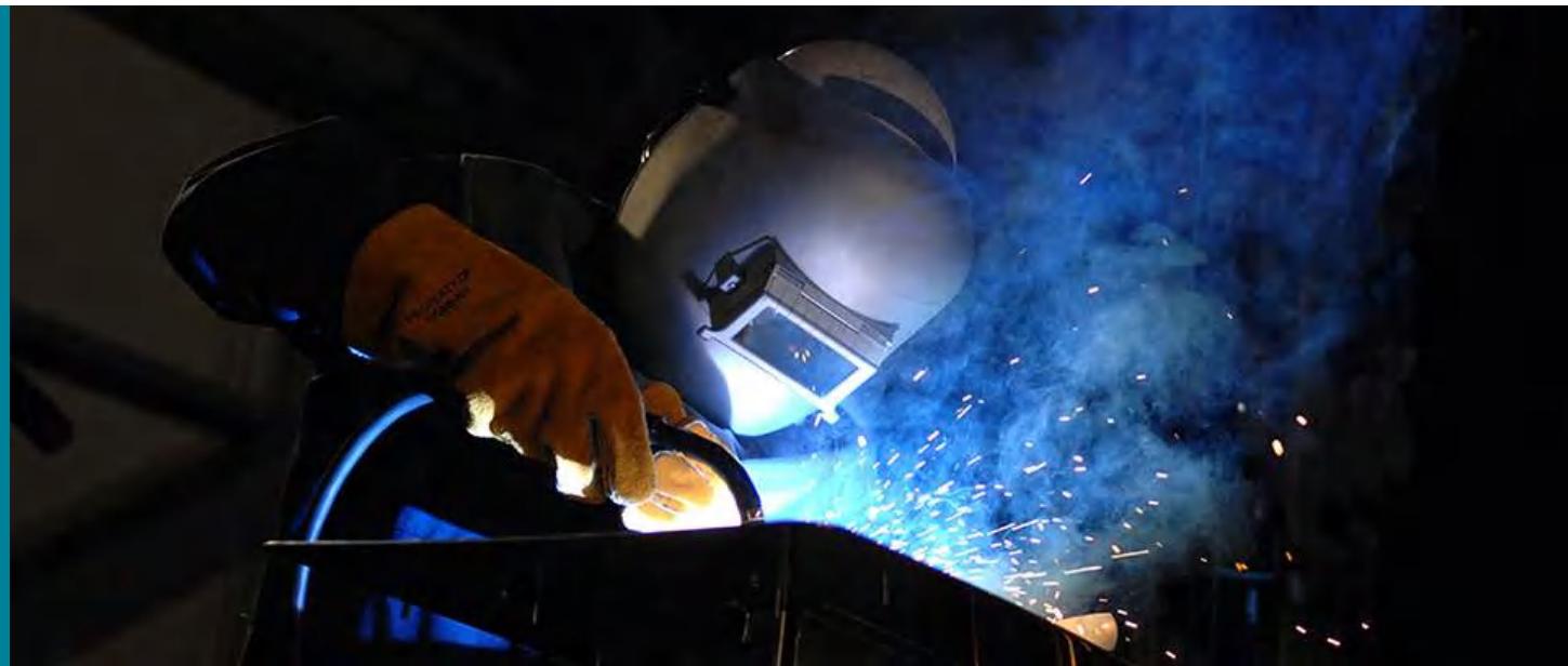
Figure 11.1 The welder's gloves and helmet protect the welder from the electric arc, which transfers enough thermal energy to melt the rod, spray sparks, and emit high-energy electromagnetic radiation that can burn the retina of an unprotected eye. The thermal energy can be felt on exposed skin a few meters away, and its light can be seen for kilometers (Kevin S. O'Brien, U.S. Navy)
