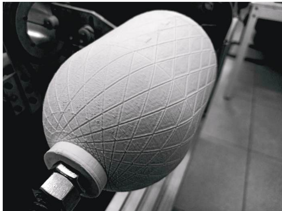
Figure 2. The mandrel with imprinted geodesic path.
