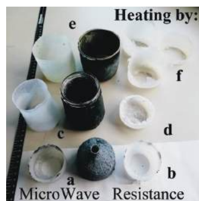
Figure 1. The PE products of molding tests and respective molds (in the between): a, c and e from the MW heating of coated AL, GL and SS molds, respectively; b, d, and f from the resistance heating the corresponding molds.
