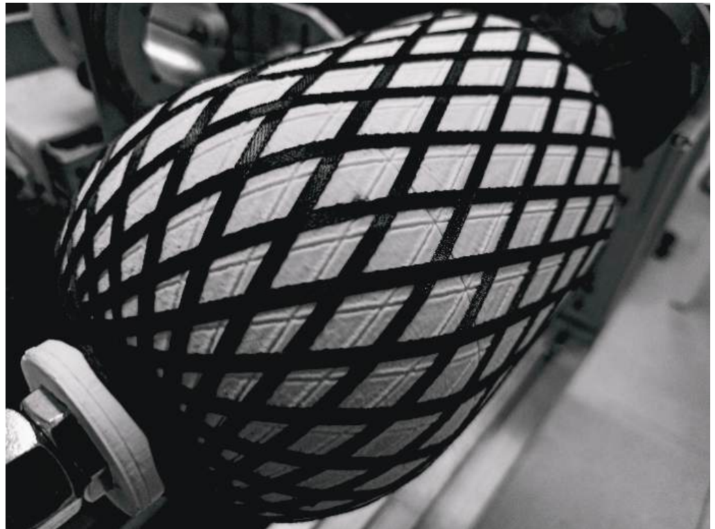
Figure 14. Wound pattern on the surface of the mandrel with the imprinted geodesic path.
