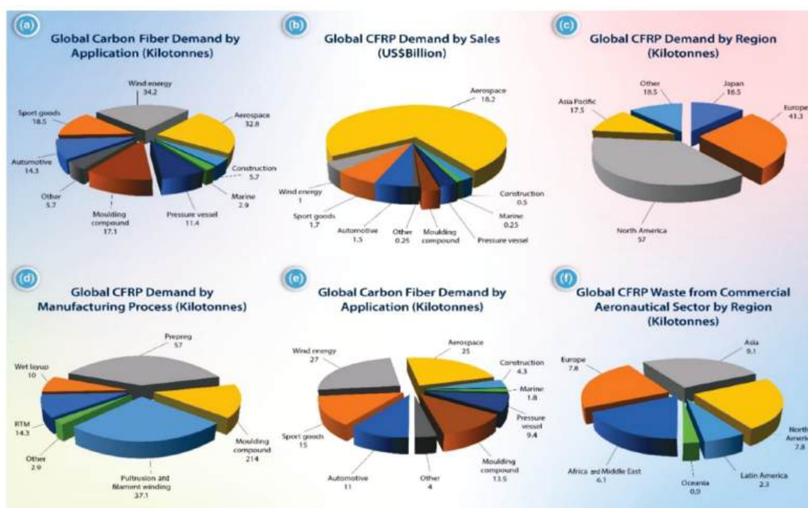
Figure 1. Global CFRP consumption in 2018 is categorized by (a) application, (b) sales, (c) region, and (d) manufacturing techniques. Global CF consumption in 2020 (e) by application and (f) estimated worldwide CFRP waste in 2050 from the aeronautical sector by region [6].
