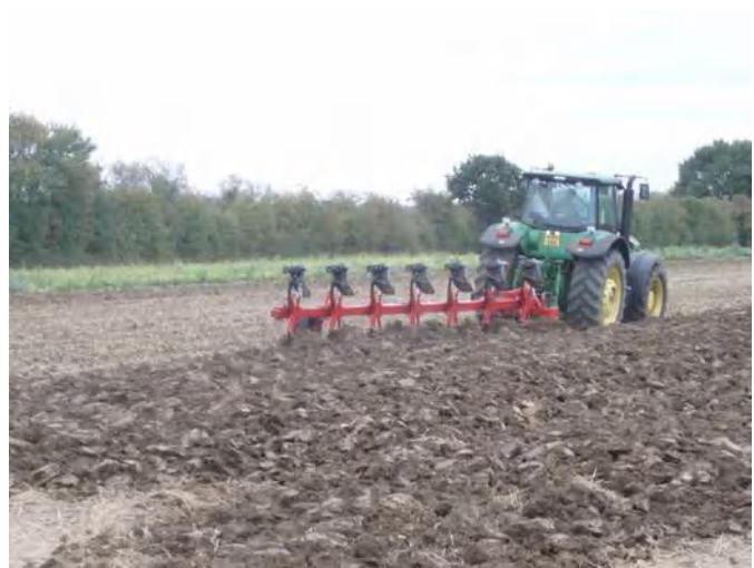
Figure 13. Tractor-mounted moldboard plow working in the field.
