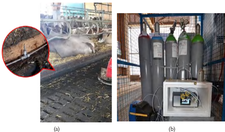
Figure 8. (a) Tracer-gas dosing by steel tubes with critical orifices protected by steel elements next to the floors in a dairy housing; (b) gas bottles with mass-flow controller.
