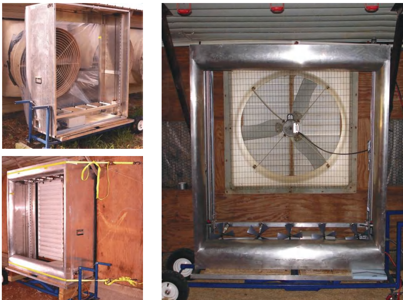
Figure 10. Fan assessment numeration system (FANS) developed by Gates et al. (2005) to describe the performance curve of a ventilation fan in an animal house. The unit can be used on either the inlet or exhaust side of the ventilation fan.
