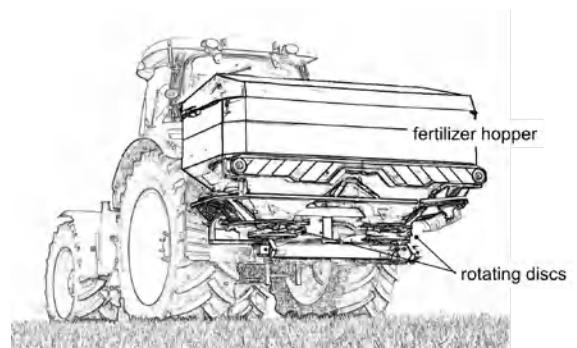
Figure 19. Centrifugal fertilizer spreader mounted on the three-point hitch of a tractor.
