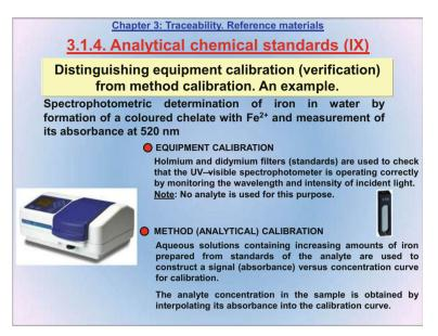
The following example distinguishes equipment calibration from method calibration with the spectrophotometric determination of iron in water by formation of a coloured chelate.
