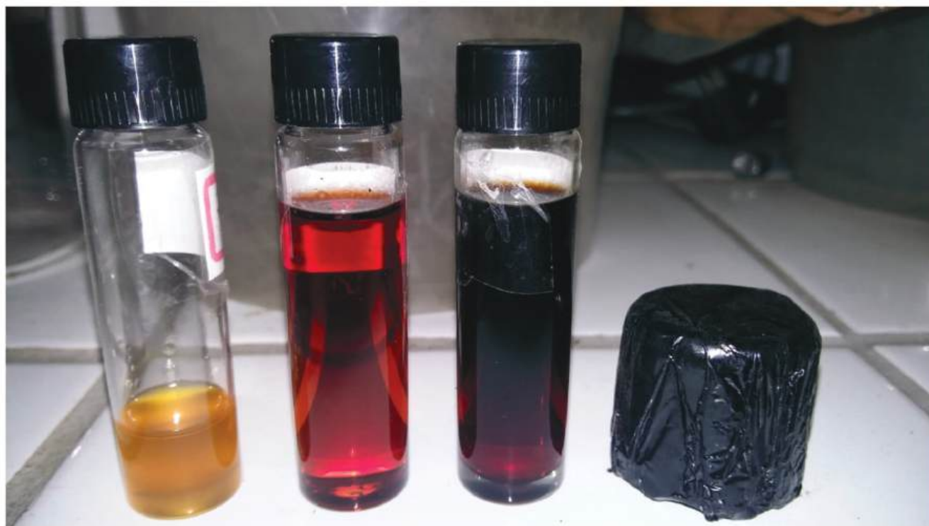
Figure 9. Distillation fractions [gasoline (yellow), light kerosene (red), and kerosene (red dark)-like boiling range temperature fossil fuels] and bottoms [Raffinate (black solid)] obtained by fractional distillation of bio-oil produced by pyrolysis of Açaí ( Euterpe oleracea , Mart.) seeds at 450 °C and 1.0 atmosphere, in pilot scale.
