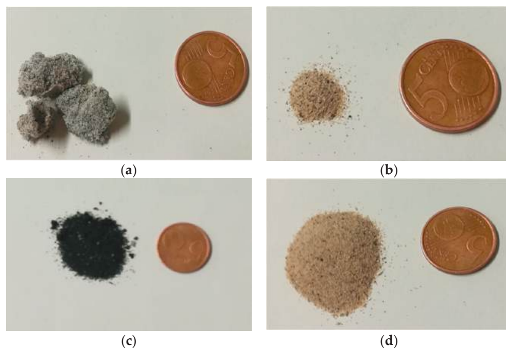
Figure 3. Examples of samples from the spent bed after the devolatilization tests: (a) coarse agglomerates of the bed, (b) top of the bed, (c) bottom of the bed, (d) intermediate part of the bed.
