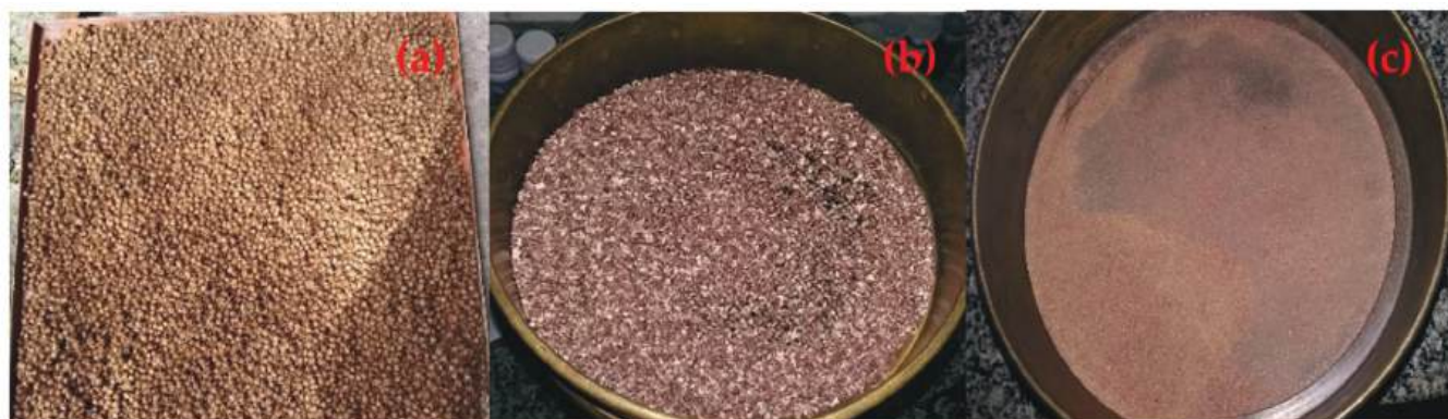
Figure 2. Material after drying, milling, and sieving process of Açaí seeds (seeds + fibers (a); comminuted seeds + fibers (b); and sieved seeds (c)).
