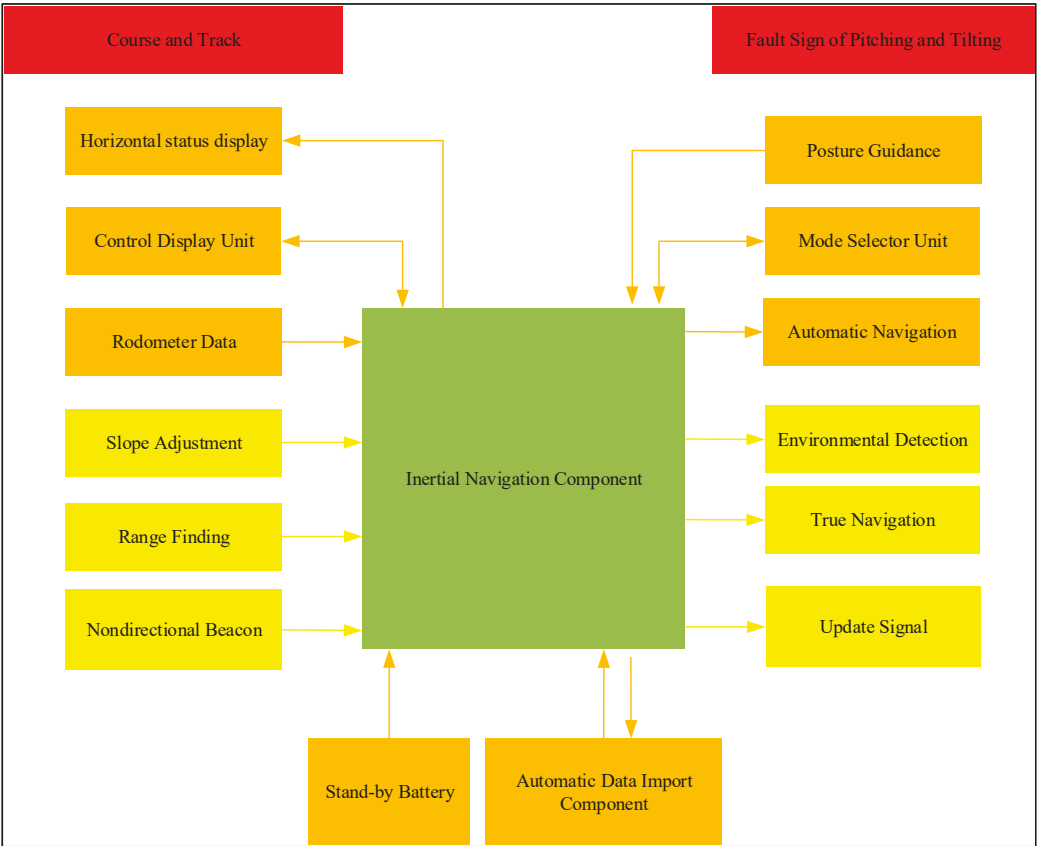
Figure 3. Structure diagram of the Inertial Navigation Straight Finding System.
