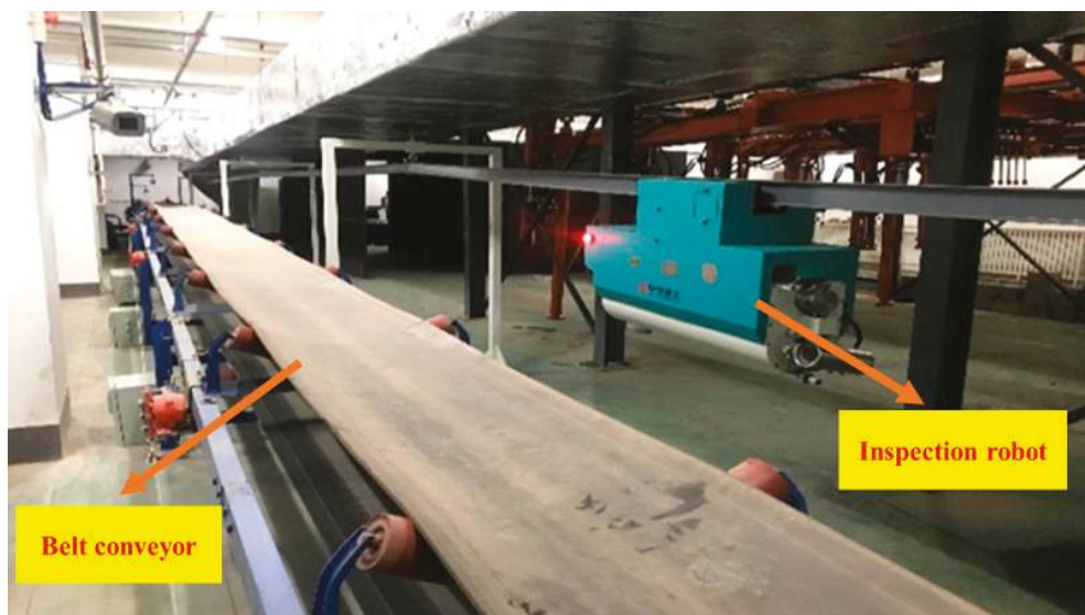
Figure 8. Working diagram of the underground inspection robot in coal mine.
