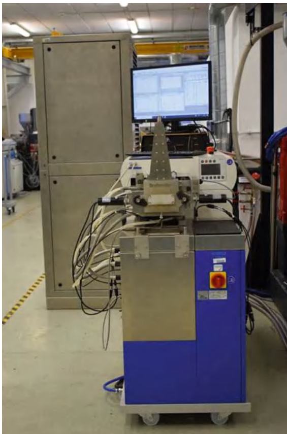
Fig. 7.4 Kneader for compounding at small scale (Source MUL facilities)
