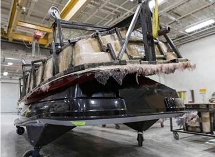
Fig. 6.83 Removing fiberglass mold from boat hull pattern (Courtesy of Thermwood)
