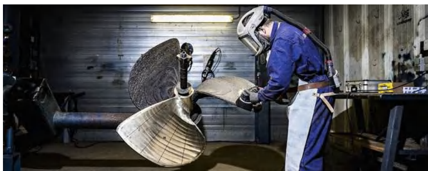
Fig. 6.76 Post-processing: grinding the WAAMPeller (Courtesy of RAMLAB)
