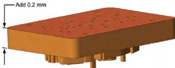
Fig. 6.10 Extension of the back face of the core/cavity (Courtesy of Stratasys)
