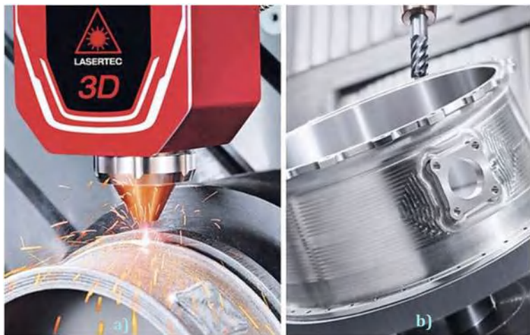
Fig. 6.20 Hybrid manufacturing process: a Laser Deposition Welding (DED), b milling (Courtesy of DMG MORI)
