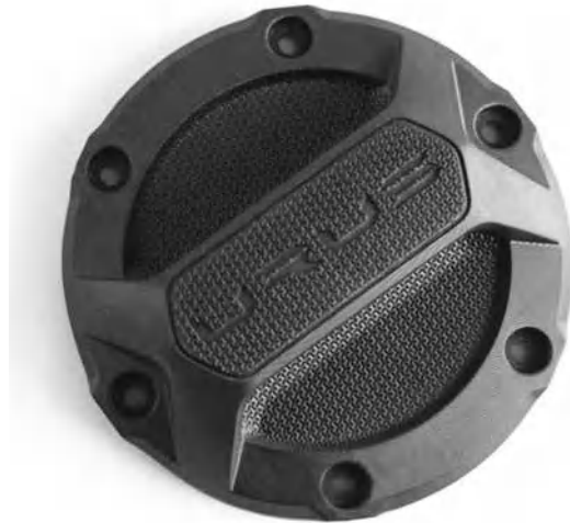
Fig. 6.100 Lamborghini Urus Fuel Cover Cap digitally manufactured in EPX 82 epoxy resin (Image credits Lamborghini)
