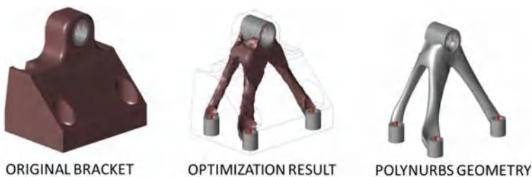
Fig. 5.19 Topological optimization. Bracket for PBF-EB/M technology (Source Skin Project—AIDIMME)
