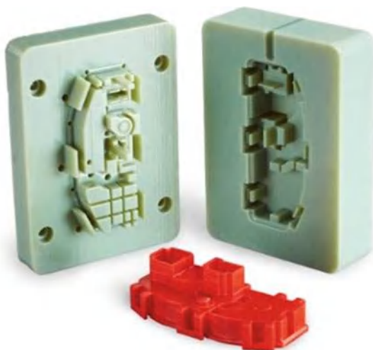
Fig. 6.2 An example of AM PolyJet (bridge) mould (Courtesy of StratasyS)
