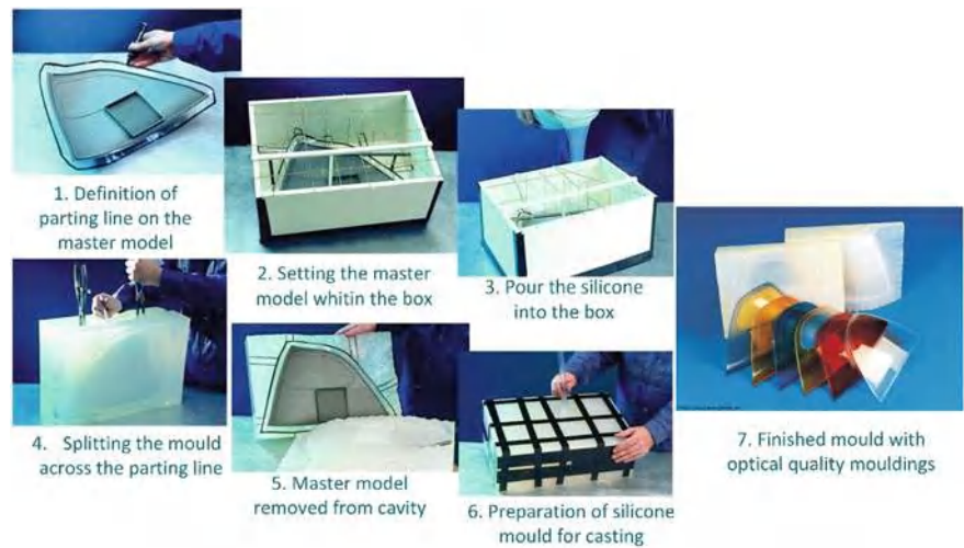
Fig. 6.5 Production process of one-piece silicone mould ( www.scott-Am.com , Courtesy of Ronald Simmonds, photographer Giulio Coscia)
