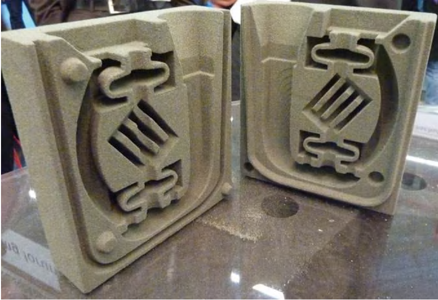
Fig. 1.17 Sand moulds made with binder jetting (Photo by Ana Pilipović)
