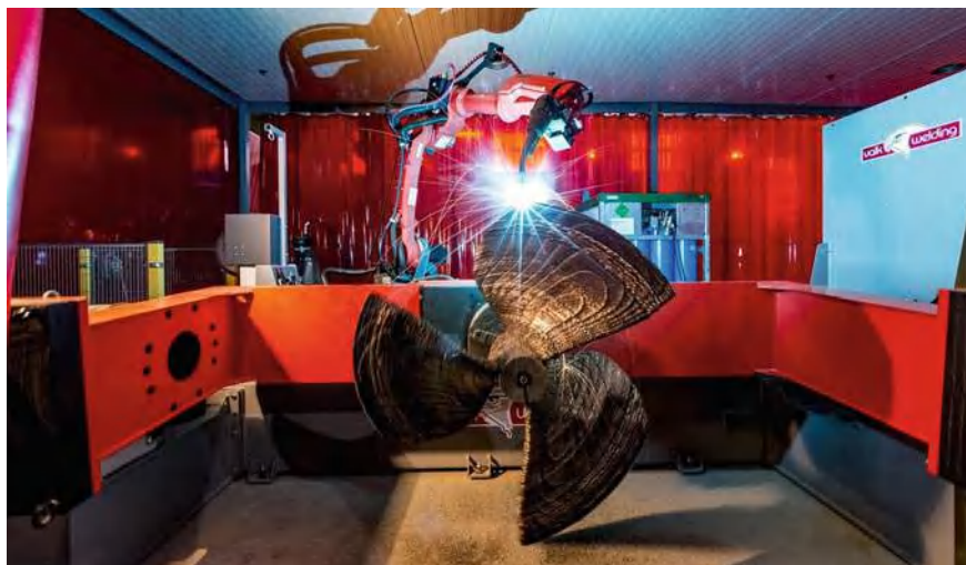
Fig. 6.75 Manufacturing of the WAAMPeller (Courtesy of RAMLAB)
