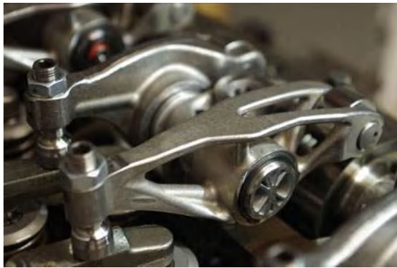
Fig. 6.102 A rocker arm manufactured by 3D printing on a bench test inside a Euro 6 engine (Image credits Renault)
