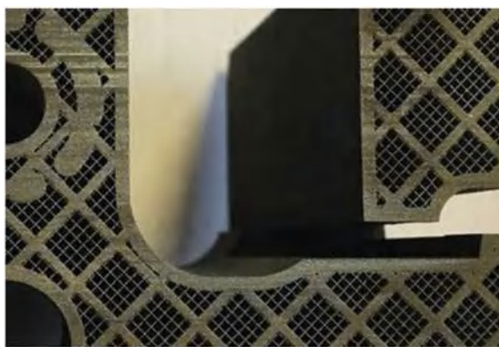
Fig. 6.39 Honeycomb structure used on inside of sheet metal tool to reduce its print time and cost (Courtesy by Olaf Diegel)
