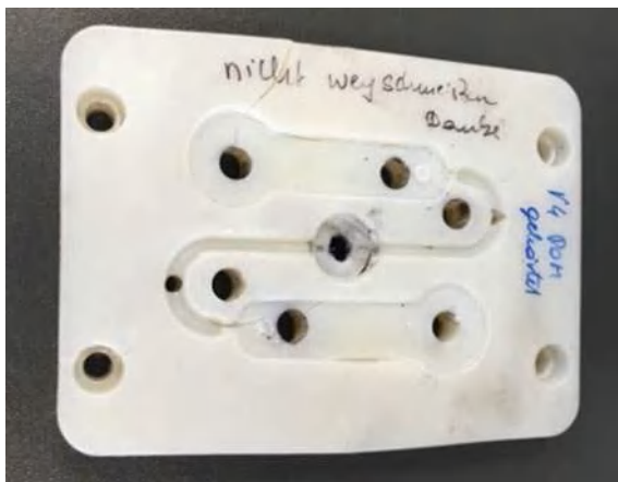
Fig. 6.18 PolyJet mould plate with cracks (Photo by Damir Godec)
