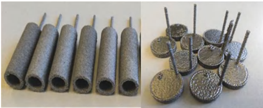
Fig. 7.44 Example of visual inspection defects (Source AIDIMME)
