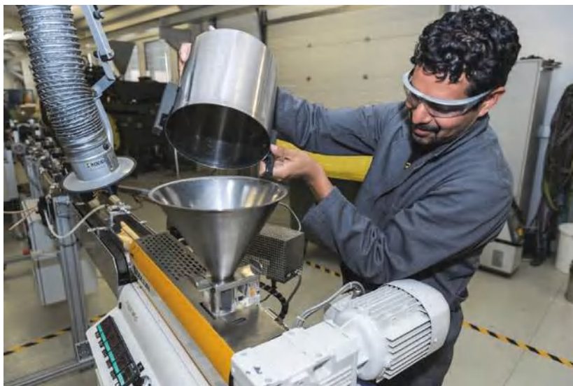
Fig. 7.13 Filament extrusion line for large amounts: a schematic (courtesy of Damir Ciglar), b real line (Source MUL facilities)
