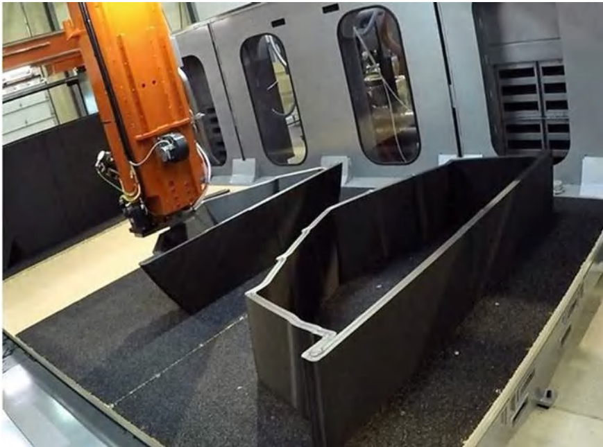
Fig. 6.81 Thermwood LSAM (3 m × 6 m) machine printing two of the six sections (Courtesy of Thermwood)
