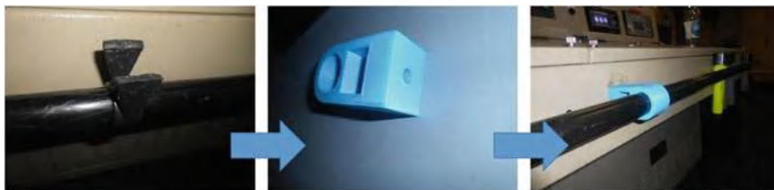
Fig. 6.90 Rail bracket replacement, 3D printed and installed on board (Courtesy of Maersk Tankers and Green Ship of the Future)
