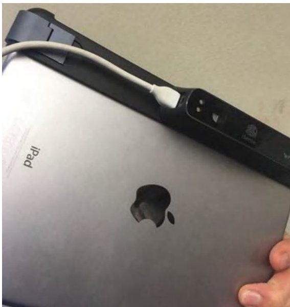
Fig. 5.25 An iSense scanner attached to an iPad (Courtesy of Per Kristav)
