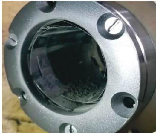
Figure 12. Disassembled bearing after maximum loading.
