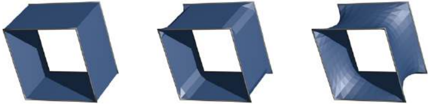
Fig. 4.2: From left to right: initial surface (512 faces); surface after a single explicit Euler step in negative discrete mean curvature direction; surface after a single explicit Euler step in negative discrete pseudogradient direction.
