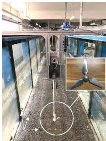
Figure 5. Layout of circulation pool and turbine.
