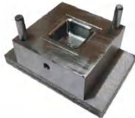
Figure 11. Bottom Die with Plate.
