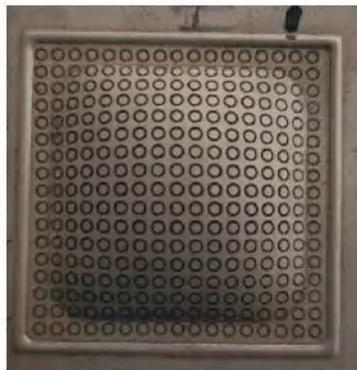
**Figure 16.** Deformed Nimonic 90 sheet for optimized parameter.
