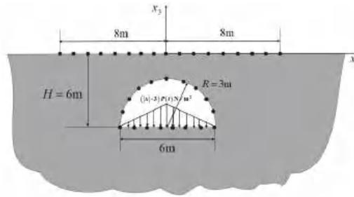
Figure 10. Schematic sketch of the semi-infinite domain tunnel.
