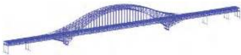
Figure 3. FE model of Guangzhou Mingzhu Bay bridge.
