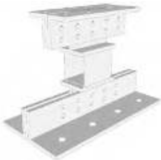
Figure 1. Schematic diagram of shear square section steel tube damper.
