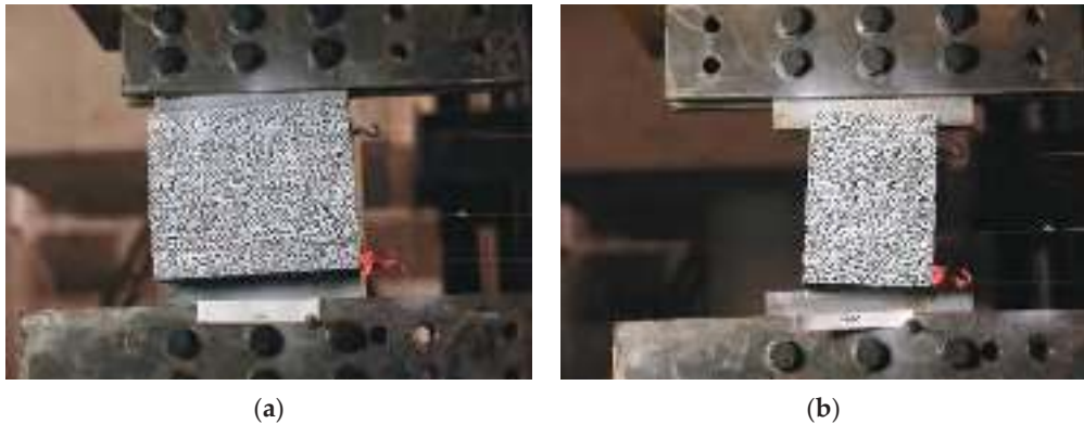
Figure 7. Failure modes of the welded steel tube dampers: (a) steel tube end of 150-C3 tearing; (b) weld of 200-A1 cracking.
