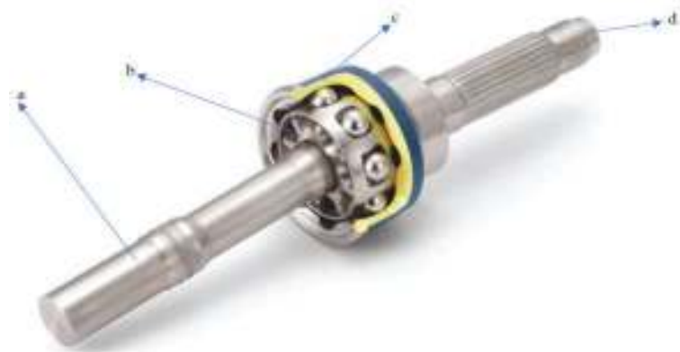
Figure 4. Details of the bowl–inner race (inner race fixed by splines on the midshaft) joint.
