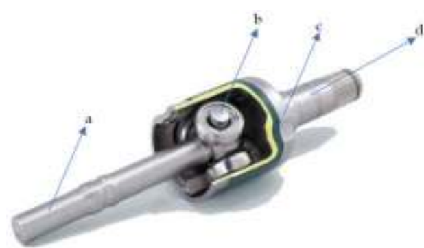
Figure 3. Details of tulip-tripod joint (tripod fixed by splines on the midshaft).
